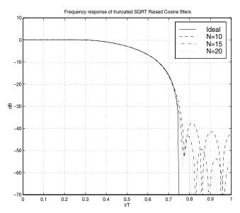
As we see, there is no significant difference in the passband area of the filters, but the realizable, truncated filters do have spectral sidelobes outside their  $(1 + \beta)/T$  nominal bandwidth. Still, depending on how much residual ISI an application can tolerate, even the N = 10 filter appears an acceptable approximation of the ideal (non-realizable) square-root raised cosine filter.
